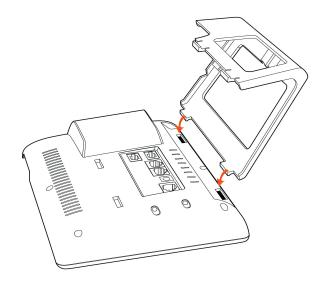
B. Press the other side joints into the slot according to the direction of the arrow:
