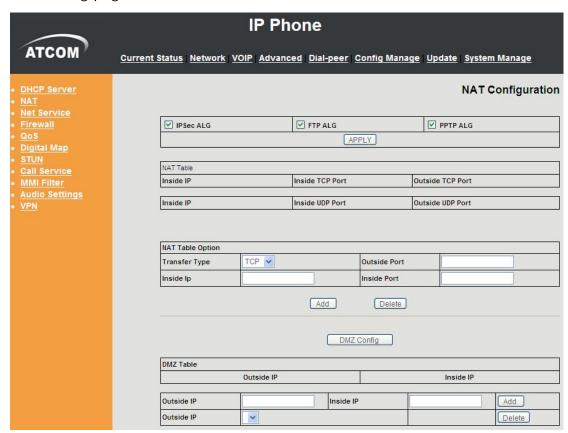
✓ IPSec ALG: It is an encryption technology. Select it to enable IPSec ALG, the
