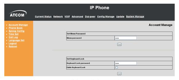
Users can add new account or delete and change existing account Set Menu Password: Set menu of keypad password, default is "123" Set KeyboardLock: The default password is "123". It will take effect when you enable the keyboard lock. The default setting is unlock, if you press any key at this status, the system will remind you to input password
