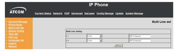
Multi line function is SIP1 or SIP2 is busying, but SIP2 or SIP1 can get the calling when have new calls with line.
