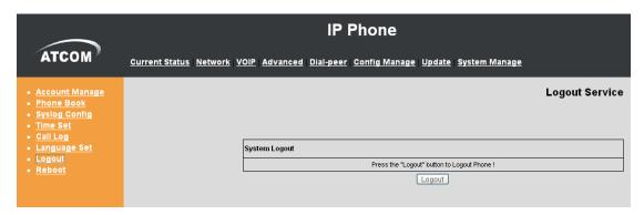
Log out the configuration mode. If you want to re-configuration the phone, need to input the user and password to login again.
